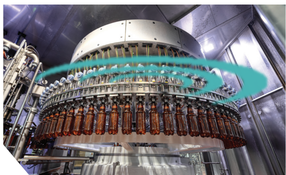
Real-time Wireless control & monitoring on rotating components
