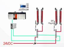
CIP Safety over EtherNet/IP enables Premier Integration of the 450L GuardShield Light Curtain in a GuardLogix® Control System and drives attachment through Smart components.
