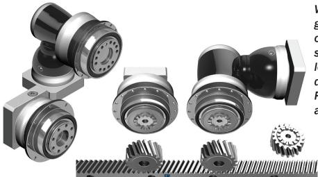
With the addition of a hypoid right angle gear set, the APK/APCK Series provides a compact, high precision right angle solution. An incredbile 1.2 arc-minute or lower backlash is standard for all ratio designs - single, double and triple stage. Ratio availability increases up to 5500:1 and torque capability to 14,000 Nm.
